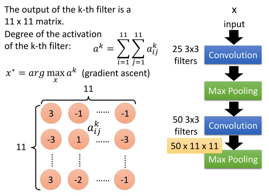
The output of the k-th filter is a 11 x 11 matrix.
