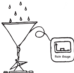
Figure 3: Rain gauge: defines "rain" as precipitation amount \geq 0.1\text{mm} .
