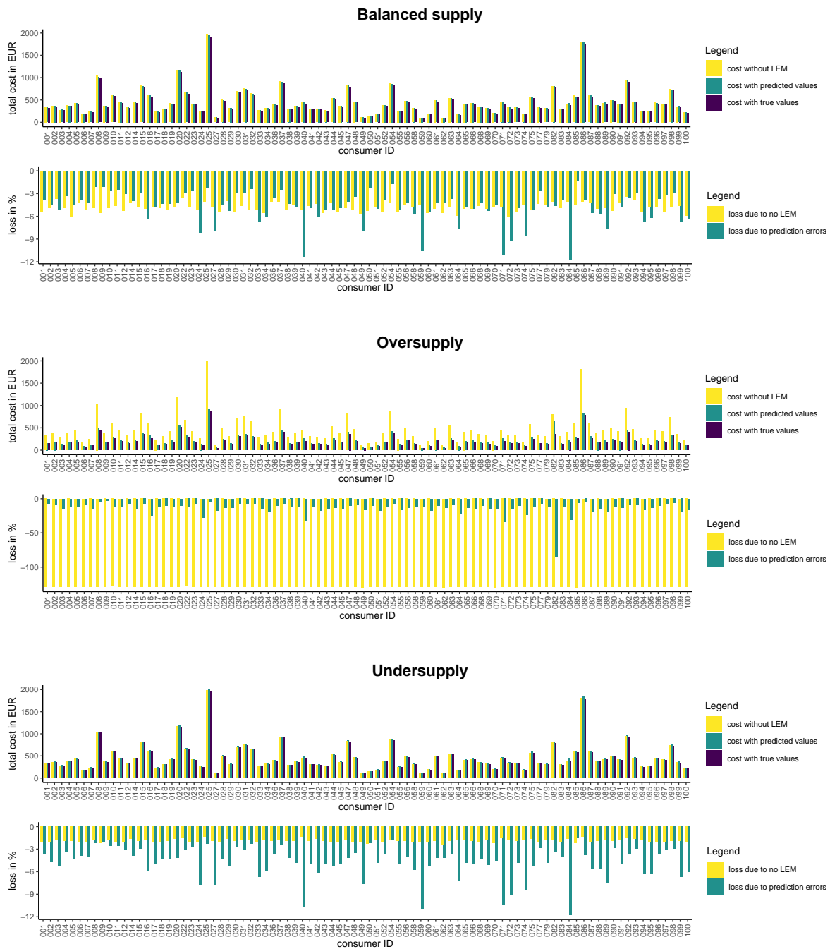
Figure 6. Total energy cost to consumers from 01.10.2018 to 31.12.2017 in case of no LEM, LEM with true values, and LEM with predicted values in three different supply scenarios. BLEMevaluateMarketSim
