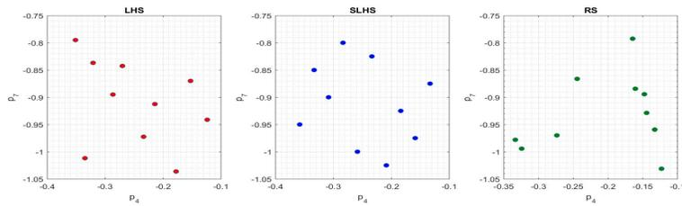
**Fig. 1** Comparison of various sampling techniques.
